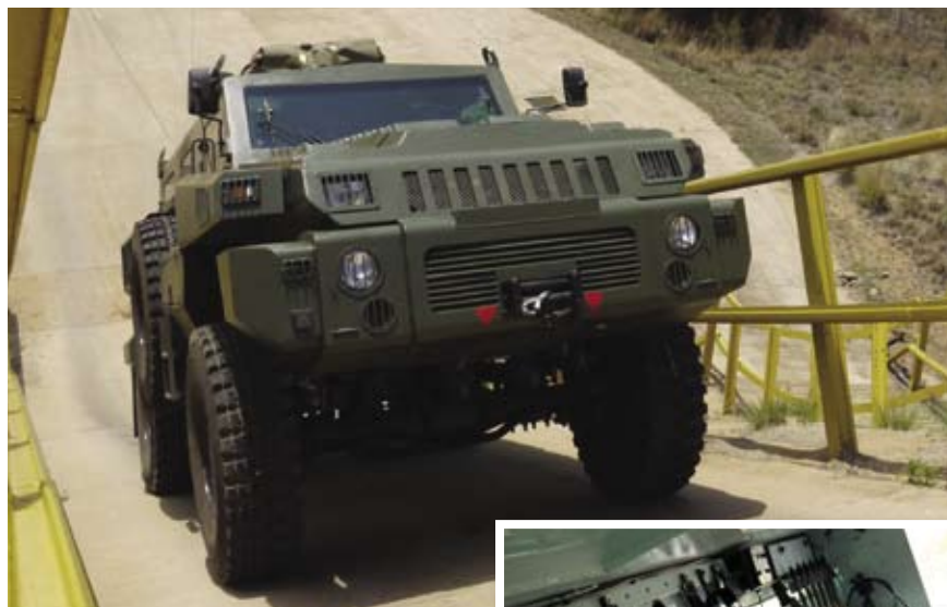
ABOVE Marauder MPV uses the same power pack and driveline as Matador but is slightly more compact RIGHT In addition to a crew of two, Marauder carries eight troops, seated on individual anti-mine seats
