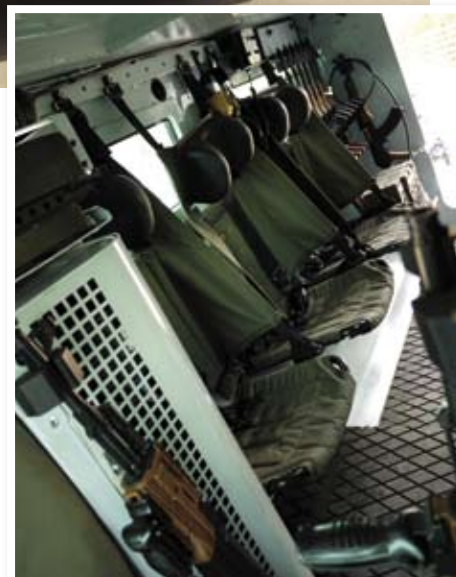
ABOVE Marauder MPV uses the same power pack and driveline as Matador but is slightly more compact RIGHT In addition to a crew of two, Marauder carries eight troops, seated on individual anti-mine seats
