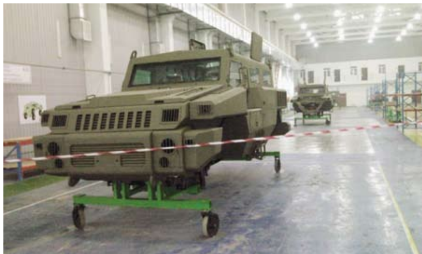
ABOVE Marauder MPV hulls work their way down the MODIAR production line in Azerbaijan
